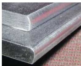
Radiusing on one or both edges. 2 - 6mm radii.
