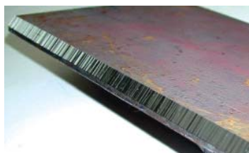
The slightly rippled bevel finish from machines with milling cutters.
