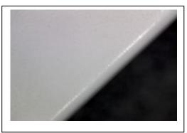
Picture 4 No corrosion on the edge of a plate which had the oxide layer removed and the edge rounded
