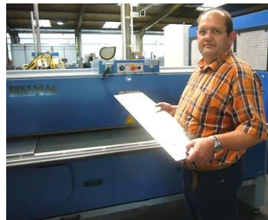
Head of Sheet Metal Processing Günther Hempfling shows that protective films remain affixed to surfaces despite grinding off sharp burrs.
