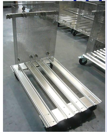
The SBM-S 1500 even removes punch burrs so perfectly that the tool cart bears no risk of cutting or quality hazards to the goods that it transports.
