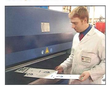
City has just installed a new £70k machine from Lissmac in Germany, the first of its kind they have manufactured. This machine will, in one pass of the blank, remove needles (or other burrs from punching or guillotines) and then polish all edges, including holes and cutouts on one or both sides. If the blank is protected with polycoating, this will be entirely unaffected by the process (provided laser quality coating is used). The unprotected side will have a fine polished finish.
