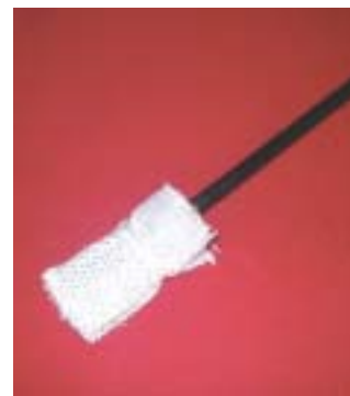
Standard paddle head with connection to handle (for cleaning with glass fibre pad)
