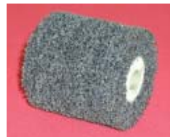
ROTO STRIP Coarse abrasive non-woven Sic mineral. 100mm OD x 100mm wide Grit: Coarse only. Bore: 19mm keyway only. Fits on to extension spindles.
