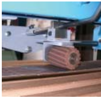
Manual operation with contact wheel. Optional pneumatic pressure assist
