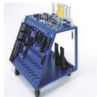
The optional tool stand with some of the most popular clamps, stops, clamping bolts, etc.
