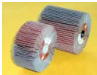
ABRASIVE CLOTH FLAP WHEELS Can be used instead of belts. Less aggressive. 100mm OD x 100mm wide 100mm OD x 50mm wide Grits: 40 - 240. Bore: 19mm keyway or 25mm round.
