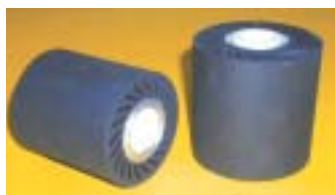
ROTO-X-WHEELS Expanding contact wheels. Expanding contact wheels are available in one hardness only. Used with abrasive belts, they are the most aggressive tools for Roto-Sat machines. Wheel size: 90mm OD x 100mm wide or: 100mm OD x 100mm wide How to mount: Fits on to extension spindle. Belt size: 100mm x 280mm (for 90mm x 100mm wheel) 100mm x 316mm (for 100mm x 100mm wheel)
