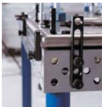
Stops set up for mitred tube.
