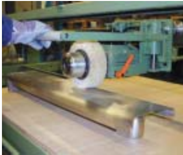
Manual operation with polishing buff
