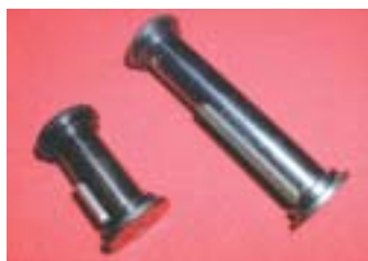
EXTENSION SPINDLES With M14 bore. 19mm dia keywayed 50mm and 100mm long. Screw straight on to the M14 spindle of the electric angle grinder.
