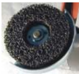
ROS Coarse abrasive impregnated nylon discs.
