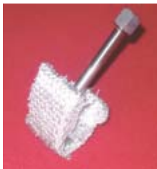
Optional corner head with connection to handle (for cleaning with glass fibre pad)
