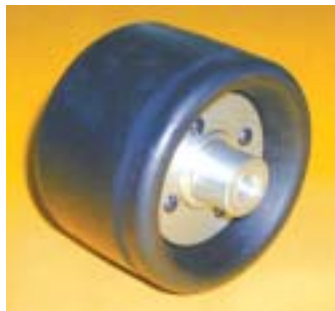
ROTOCUSHION 120 Pneumatic contact wheel. Wheel size: 120mm OD x 80mm wide. How to mount: Screws straight on to M14 spindle. Belt size: 90mm x 395mm.
