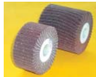
ROTO COMBI Mixed abrasive non-woven and abrasive cloth. 100mm OD x 100mm wide 100mm OD x 50mm wide Grits: 60, 80, 120, 180, 240. Bore: 19mm keyway or 25mm round. Fits on to extension spindles.
