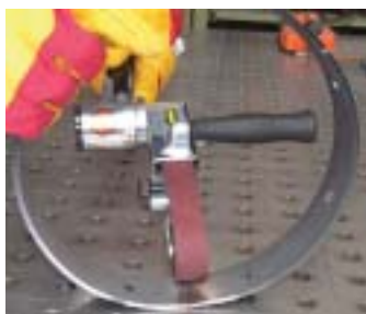
Model 620 grinding a weld inside a ring.
