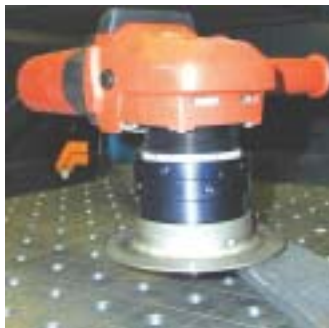
The milling head for Model 2014-R milling machine with 3 carbide inserts.
