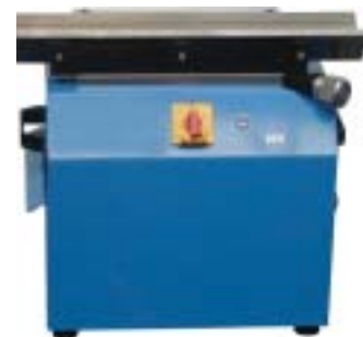
0 - 10mm chamfer (horizontal cutting head)
