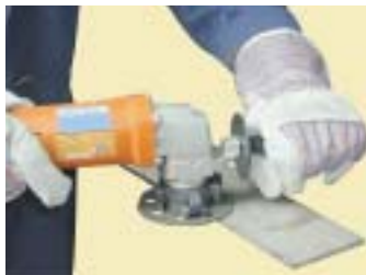
Model ASO 314 Portable Milling Machine For bevels up to 3mm wide. 45° angle only. For straight & contoured edges.
