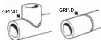
Grind and blend fillet welds
