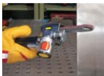
Model 610 air belt file deburring a sheet edge
