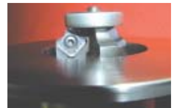
The milling head for Model 2014-R milling machine with 3 carbide inserts.
