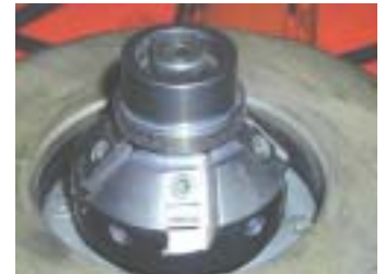
The milling head for our top of the range radiusing machines. With 5 carbide inserts.
