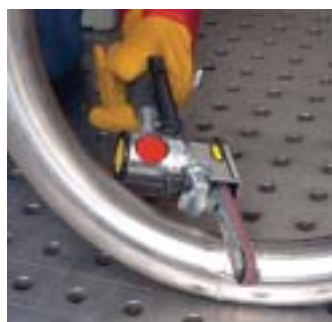
Model 610 air belt file polishing a weld on a tubular ring
