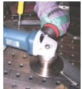
The milling head for Model 2014-R milling machine with 3 carbide inserts.
