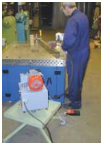
Roto-Flex in action graining hollow sections.
