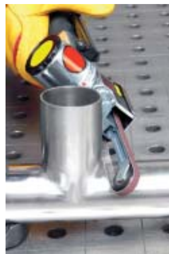
Model 610 air belt file blending a fillet weld
