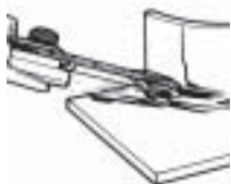
Grind and blend fillet welds
