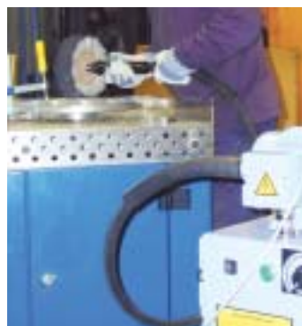
Roto-Flex in action polishing a wheel.
