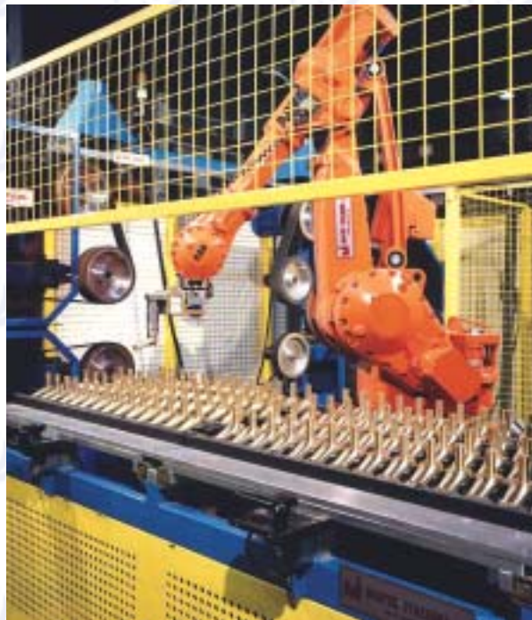
1 off MAPOS robot cell for finishing and polishing brass taps.
