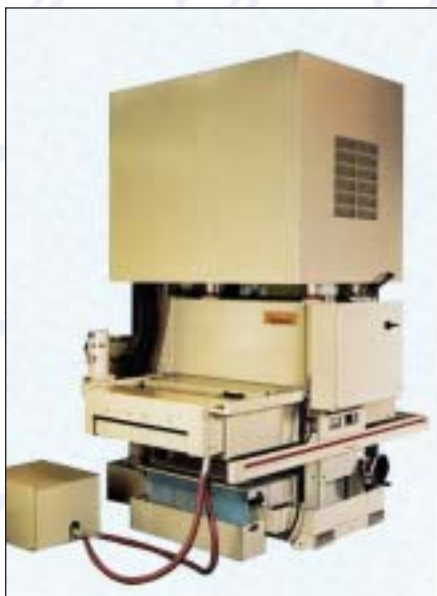
1 off Timesavers abrasive disc machine, model CS 360 for deburring clad aluminium sheet. Wet operation including drying unit.
