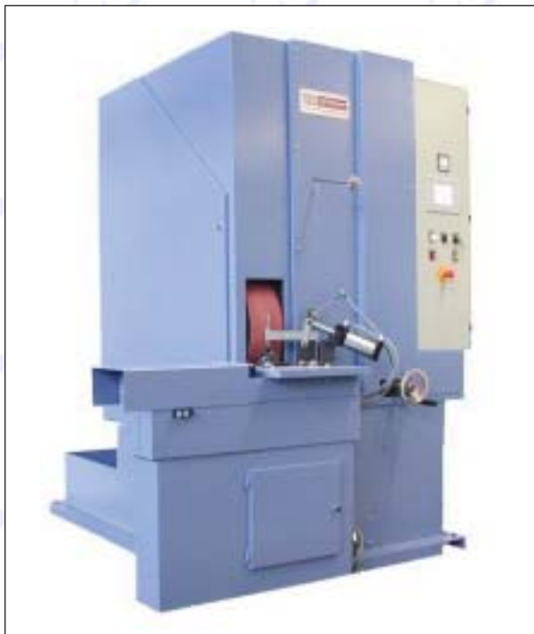
2 off Reichmann abrasive belt power grinders with vertical table and incremental feed.
