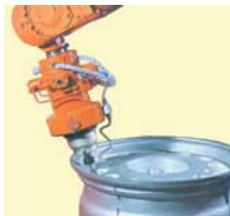
Robot deburring an alloy wheel
