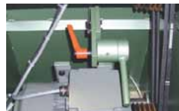
The quick change, 3 speed pulley / v-belt transmission
