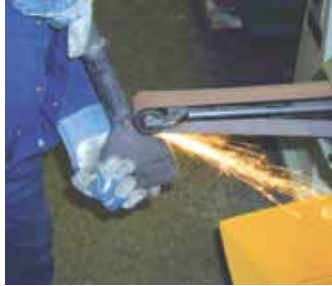
Model 491 in action. With 50mm dia contact wheel and extended belt arm. Large dust capture hood.
