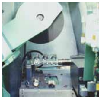
Cutting head in position for vertical stroke. Table horizontal.
