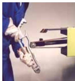
Model 706 in action. Fitted with 50mm dia contact wheel. No side restrictions.
