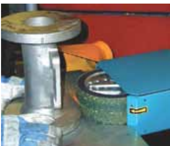
Model 127 in action. Removing the flash line on the outside diameter of a round casting.
