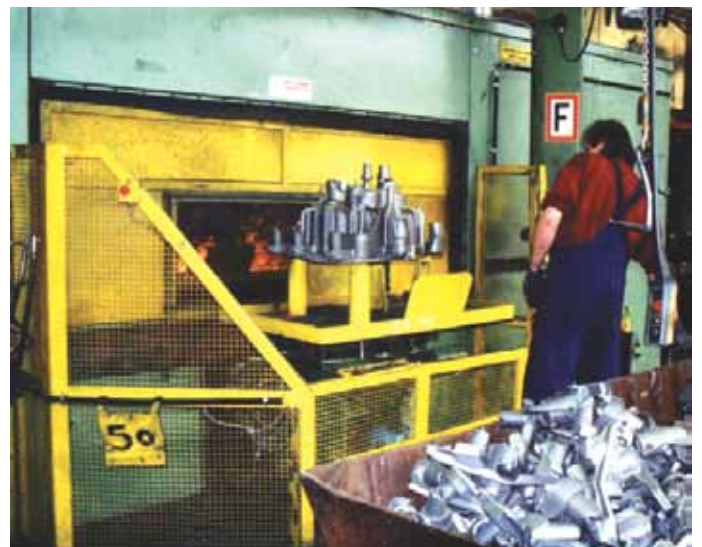
Model TS600-S90 in action. Whilst the operator loads and unloads one pallet, another is inside the machine and the casting is cut as programmed
