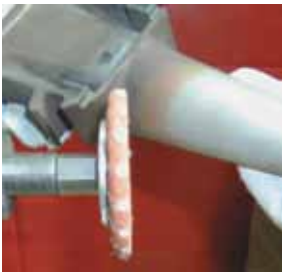
Finishing difficult areas with Sandex abrasives.
