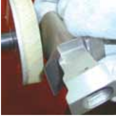
Superfinishing turbine blades with diamond brushes.
