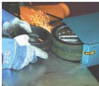
Model 127 in action. Removing the flash line on the outside diameter of a round casting.
