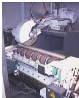
The OD grinding head and carriage inside the enclosure
