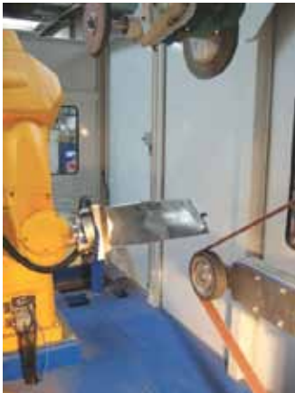
Robot finishing a turbine blade
