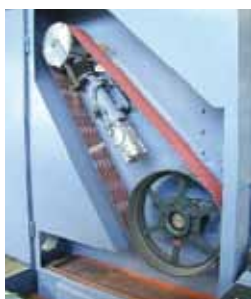
Abrasive belt head with 3500mm long belt and 500mm dia. steel face contact wheel
