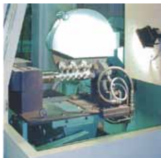
Cutting head in back position of horizontal stroke. Table horizontal.
