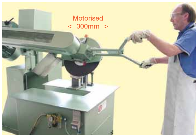
Cutting head tilts and can be moved back and forth 300mm
