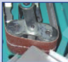
Special design abrasive belt head with oscillating contact rollers for producing a radius.
