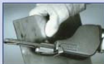
For the occasional sheet deburring, consider using a portable abrasive power tool with a special cranked arm.
