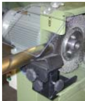
With V-guide support for deburring internal and external tube ends
