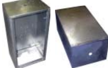
Typical welded enclosures for blending welded corners and for graining all surfaces
