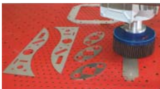
Parts as small as 50 x 50mm are firmly held in position. Perforated polyurethane mat facilitates dust extraction
