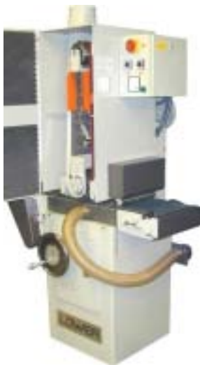
Model STN 300 with 1 abrasive belt head.
