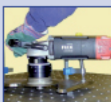
A portable radiusing machine with milling cutters to produce 2mm to 5mm radius.
