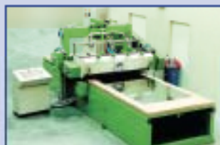
Model RON. Top class mirror polishing machine, either with reciprocating table or head.
