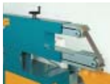
Abrasive belt can be angled to facilitate deburring action
