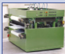
Model Combi III. For automatic marbling and application of protective tape.
