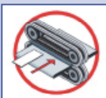
Diagram of the four counter rotating brush belts in Model SBM-S.
