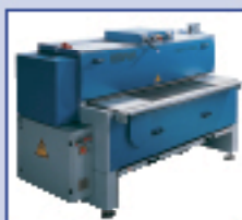
Model SBM-S Special deburring machine with four counter rotating brush belts. With two cross belts for the top side and two cross belts for the bottom side.
