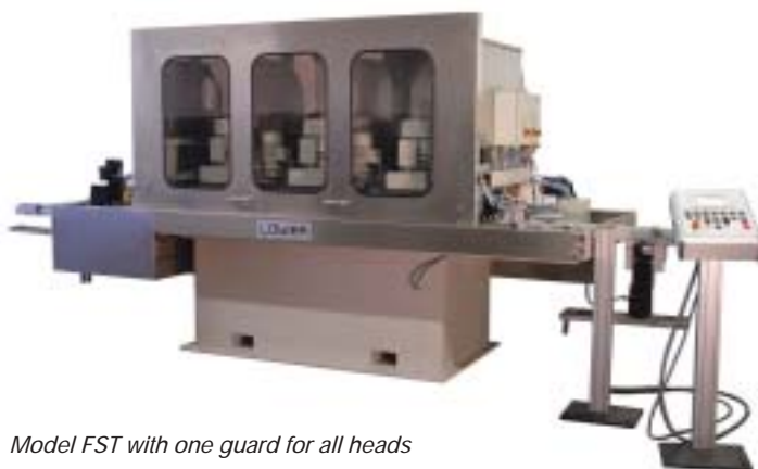
Floating heads for parts with uneven surface, ie hollow sections and some bar and plate.
