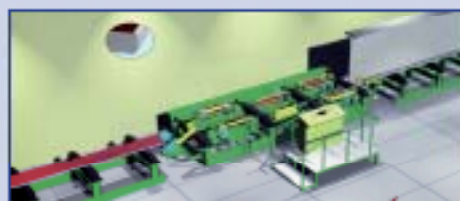
Fully automated machine for chamfering and radiusing of long parts.
