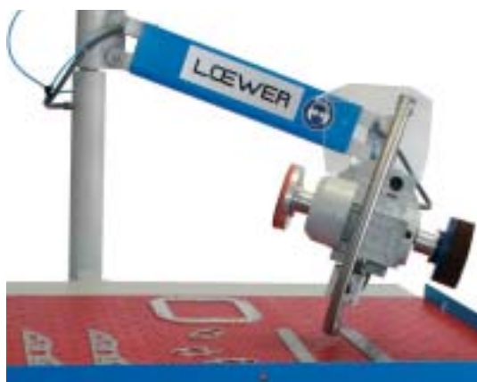
The tilting deburring head with 2 discs
