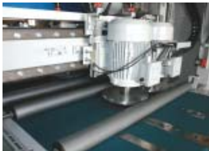
Close up of one of the two reciprocating heads.
