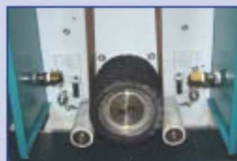
Narrow belt throughfeed machine showing contact wheel and two hold down rollers.
