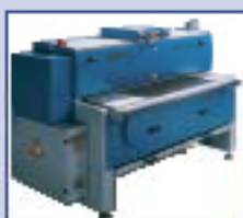
Model SBM-8 Dedicated wire brush belt machine. For removing oxide film from edges.
