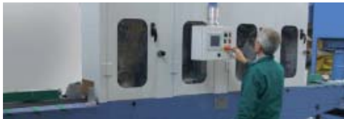
Model SP multi head with 4 abrasive belt heads and PLC control
