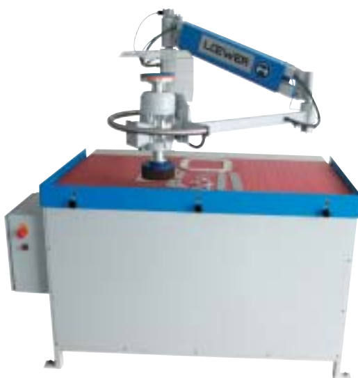
Swing grinder with weight balanced arm, tilting deburring head and large table
