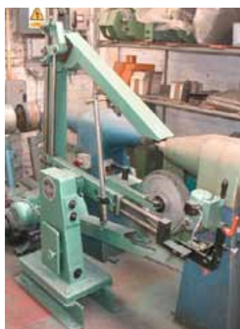
Model KS 350 Shown here with optional BC centreless attachment for grinding and polishing of tubes.
