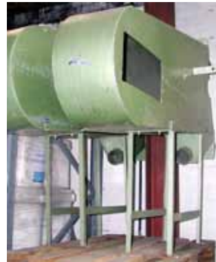
This picture shows a typical guard used for abrasive belt bench type backstands.
