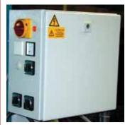
Control box for an abrasive belt throughfeed conveyor machine. With isolator switch, ammeter for contact pressure control, oscillation on/off switch, conveyor motor and main abrasive belt drive motor switches. In metal enclosure with large access door.
