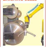
Contact wheels used with robot grinding and linishing cells are very similar to those used for manuals abrasive belt grinding and yet differ in some important details.
