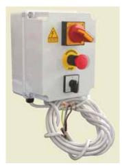
One of the most sophisticated motor control units for an abrasive belt grinding machine. With isolator, E-stop and two sped selector switch. Inside is an overload relay, a DC injection brake and room to fit extra relays to control an extractor.
