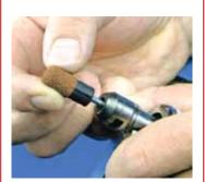
Shaft mounted rubber holders for abrasive cloth caps.
