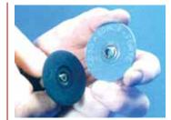
The "click on" method of fixing discs to back up pads
