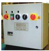
Control box for an abrasive belt tube polisher. With emergency stop, on/off push buttons, switch for main motor, switch for feed motor, isolator. Bottom left shows the variable speed control for the feed wheel motor. Inside are also overload relays.
