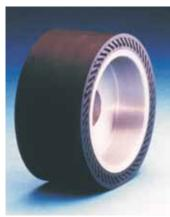
An expanding rubber wheel which allows you to turn a polishing machine without belt arm into an abrasive belt grinder.
