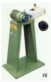
One of our standard pedestals for belt grinding and polishing machines.
