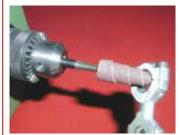
An abrasive cartridge wheel mounted on a dedicated tapered spindle and fitted to a machine with chuck.
