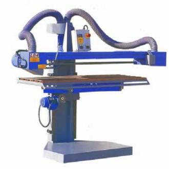
A pad sander with two spigots and flexible metal ducting joined by a Y-piece before a single flexible Duct is connected to the extractor.
