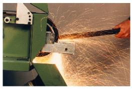
Mild steel being ground with a coarse abrasive belt.
