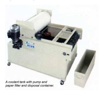
For large grinding and polishing machines with wet operation we recommend hydrocyclones. They can handle much larger amounts of coolant than coolant tanks with paper filters.
