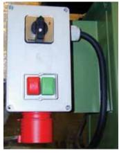
Another basic switch for a budget machine. With 2 speed selector switch, on/off push buttons and socket. Also with overload.
