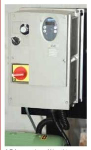
A Telemecanique Altivar 31 inverter. Programmable and with overload protection. This is the standard inverter we use unless requested otherwise.
