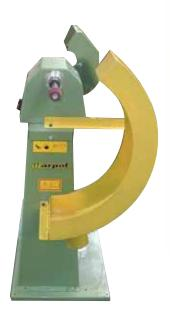
A rather special guard and capture hood. This was the only design that made the finishing operation possible. It does not fulfil all safety requirements but our customer overcame that by allowing only trained operators to use the machine.
