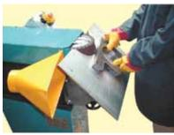
On these two machines guards and capture hoods are separate. Guards have been designed not to interfere with the grinding operation. Capture hoods are hinged and can be positioned to catch the dust from various directions.
