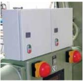
Two DOL starters, two motor brakes, overloads and two emergency stop switches fitted to a heavy duty double ended abrasive belt grinder.
