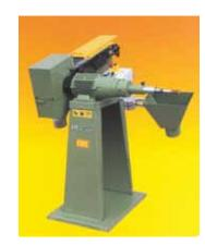
This is a milling, grinding and polishing machine for the orthopaedic Industry.
