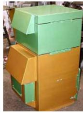
A dry extractor with explosion panel and blast barrier
