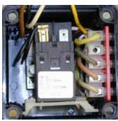
The inside of the very basic motor control. With on/off switch and thermal overload in the centre and terminal block on the right.
