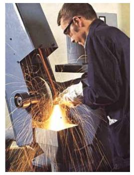
A special arrangement for large amounts of hot dust. The guard is cut back to suit the operation and a separate large capture hood with spigot is fitted to catch most of the dust. Even so, you can see that some dust and sparks escape.
