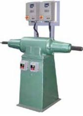
A 40 year old polishing machine with independent motors for each spindle end. Each motor fitted with frequency inverters (variable speed drives = VSD) to allow speeds between 2000 rpm and 3200 rpm to be used.
