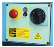
Control box for a twin speed Bench top abrasive belt grinder, incl. E-stop.
