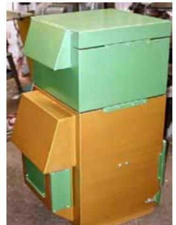
A dry extractor with explosion panel and blast barrier
