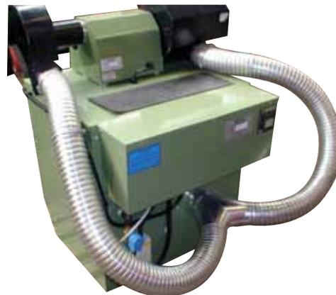
The photo shows a bench polisher mounted on a wet extractor. Heavy duty flexible ducting connects the machine with the extractor. See Y-piece used as inlet spigot. The unit is suitable for polishing titanium.
