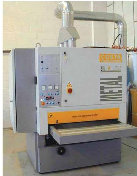
*A wide belt machine with three way manifold and smooth fixed metal ducting of 14 gauge steel.*
