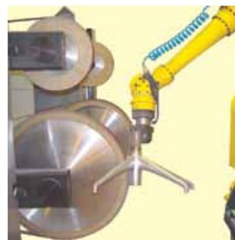
Contact wheels used with robot grinding and linishing cells are very similar to those used for manuals abrasive belt grinding and yet differ in some important details.
