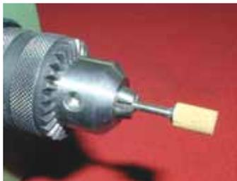
A bench grinder/polisher with a chuck fitted.
