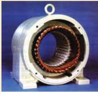
Motor housing and windings. Shown without rotor.
