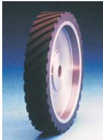
The most widely used contact wheel. Same tyre as GL but serrated to prolong belt life. Available in 40, 60 and 80 shore hardness as standard.
