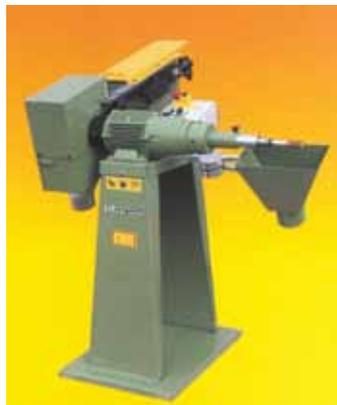
This is a milling, grinding and polishing machine for the orthopaedic industry. On the left a flatbed finishing head with standard guard. On the right a capture hood with spigot which is adjustable in all directions.
