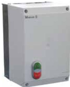
*A control box with DC injection brake, overload relay and direct on line starter control (DOL). In IP 65 GRP enclosure and with motor overload.*
