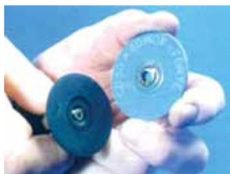
The "click on" method of fixing discs to back up pads
