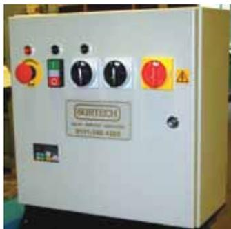
Control box for an abrasive belt tube polisher. With emergency stop, on/off push buttons, switch for main motor, switch for feed motor, isolator. Bottom left shows the variable speed control for the feed wheel motor. Inside are also overload relays.
