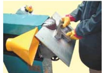
On these two machines guards and capture hoods are separate. Guards have been designed not to interfere with the grinding operation. Capture hoods are hinged and can be positioned to catch the dust from various directions.
