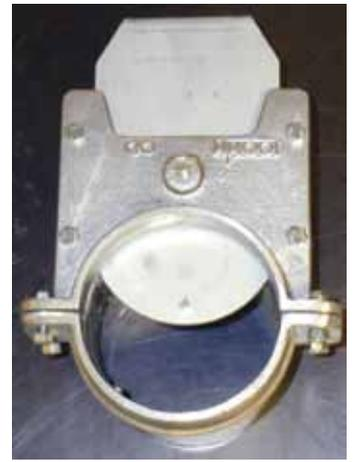
*A damper allows you to increase or decrease the airflow on each spigot*
