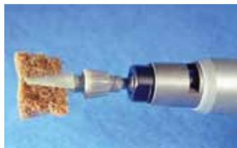
A crocodile holder mounted on a portable tool with collet and equipped with a piece of abrasive impregnated nylon.
