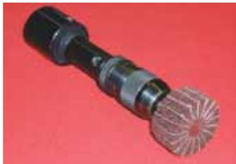
A special design shaft with threaded internal bore on one end and chuck on the other end.
