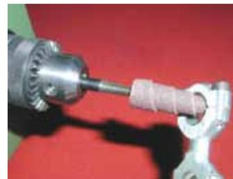
An abrasive cartridge wheel mounted on a dedicated tapered spindle and fitted to a machine with chuck.
