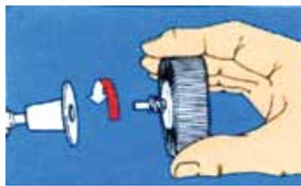
The tool holder system for wheels is very similar to that of the "twist on" disc but with an additional locating tab to make sure the wheel runs true.
