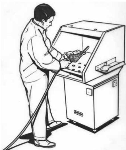
A portable abrasive belt grinder used with a bench extractor
