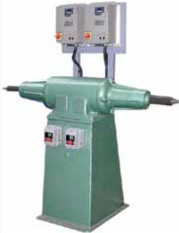
*A 40 year old polishing machine with independent motors for each spindle end. Each motor fitted with frequency inverters (variable speed drives = VSD) to allow speeds between 2000 rpm and 3200 rpm to be used.*
