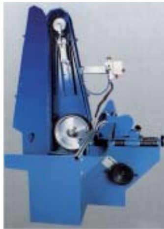
Side view with vertical belt head, contact wheel and feed wheel.
