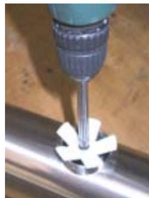
Abrasive Star disc for deburring holes or tube ends
