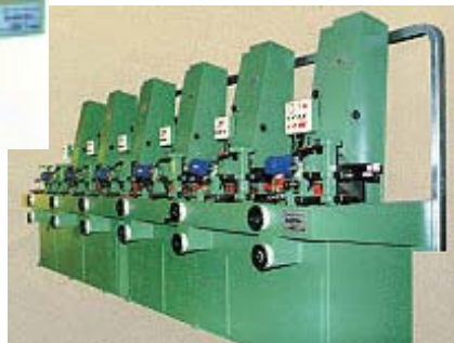
A 6 head centreless machine with vertical heads and without a conveyor system.
