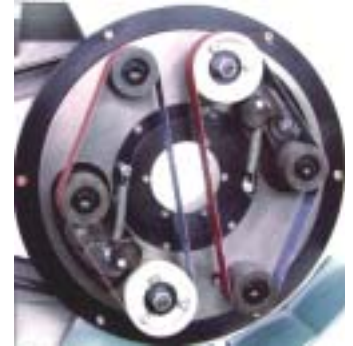
The planetary drive of a planetary tube polishing machine for diameters from 10mm to 100mm.
