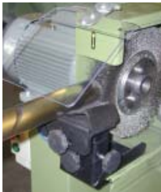
With V-guide support for deburring internal and external tube ends
