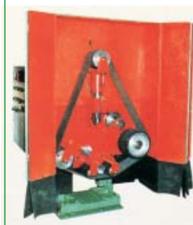
This abrasive belt head blends welds on welded tube by oscillating across the weld. The tube does not rotate.
