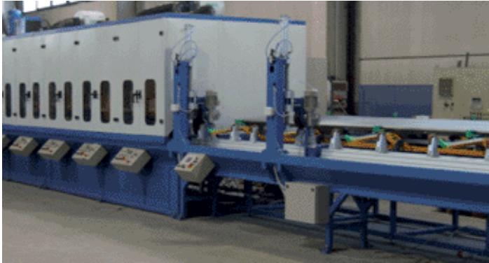
A multi head STO model, fully enclosed, with automatic loading and unloading, large roller conveyor and pinch rolls.
