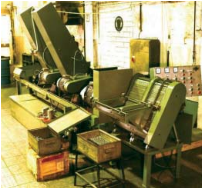
Centreless machine with 2 abrasive heads and automatic loading and unloading. For finishing of ratchet screwdriver rods.
