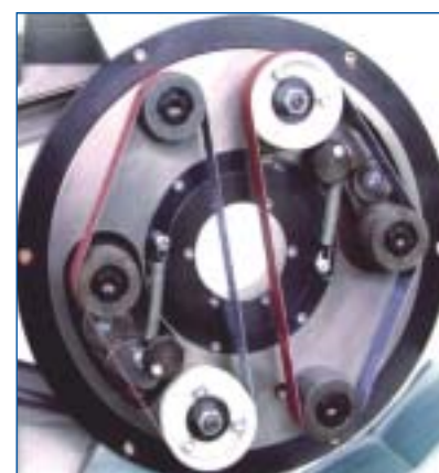
Two rotating abrasive belt heads mounted on rotating disc
