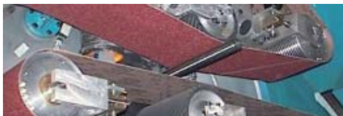
Close up of an orbital abrasive belt head. Both belts rotate around the tube.
