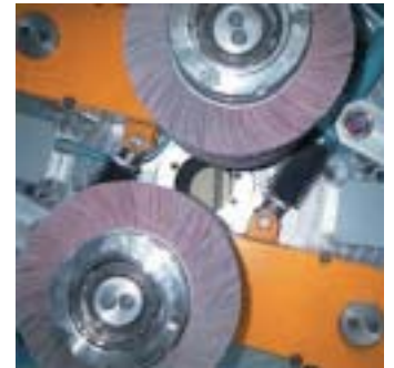
Close up of an orbital brush head. With two abrasive brushes which both rotate around the tube. The tube is fed through the hole between the brushes.
