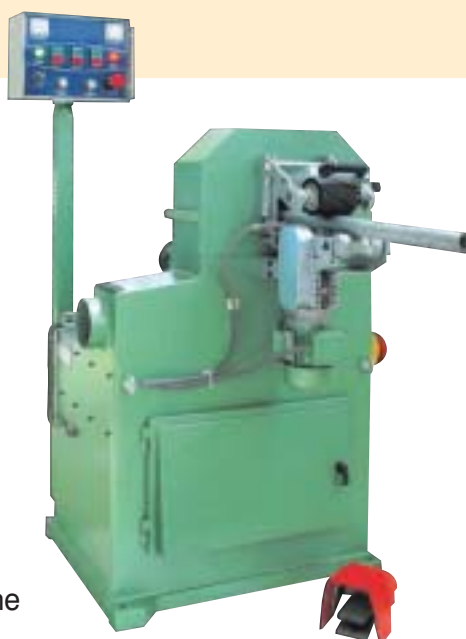
Two rotating abrasive belt heads mounted on rotating disc
