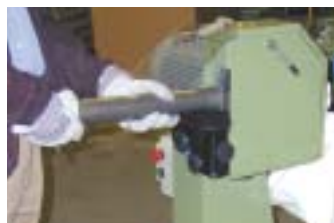
Model Surtj JT set up for deburring tubes.
