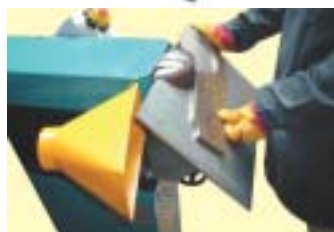
Bevel prior to welding
