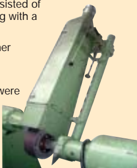
The traditional abrasive belt grinder with backstand arm mounted on the motor of a polishing lathe.
