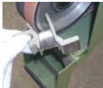
Series 7 with special contact wheel with no side restriction
