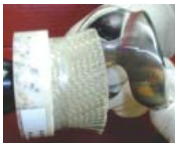
Superfinishing implants with diamond brush.
