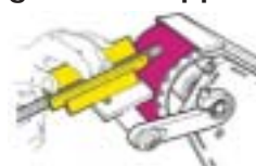
Optional SURTECH fixture for deburring tube ends
