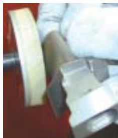
Superfinishing turbine blades with diamond brushes.
