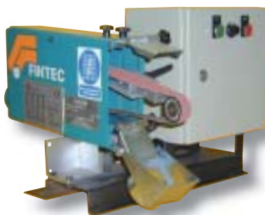
Model 411 Variable speed belt grinder. With interchangeable contact arms. Contact wheels from 15mm to 100mm dia.
