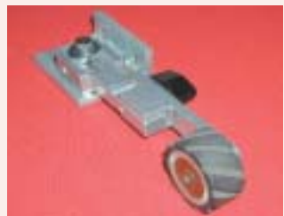
Adjustable bracket with one of the many large contact arms. Incorporating abrasive belt tracking control.
