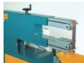
Abrasive belt can be angled to facilitate deburring action
