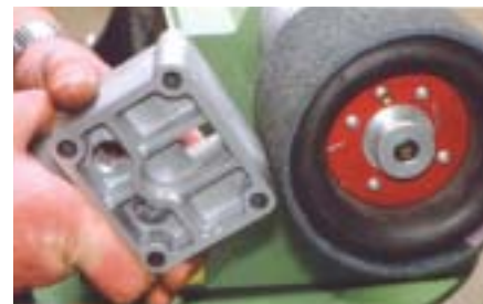
Satin finishing with abrasive nylon belts.
