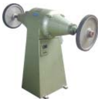
A double ended polishing lathe with contact wheels fitted. Often polishing mops were used as contact wheels.
