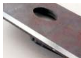
The smoothest finish produced by abrasive belts or discs.
