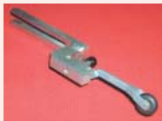
Adjustable bracket with one of the many small contact arms. Incorporating abrasive belt tracking control.
