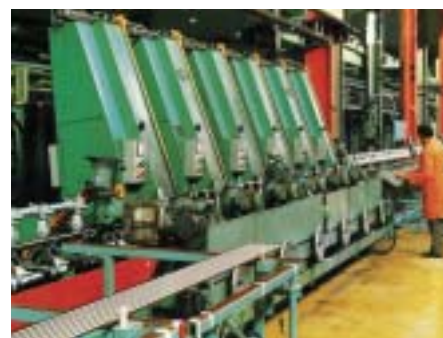
A six head fully automated tube grinder.
