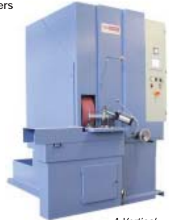
A Vertical Power Grinder removing feeders from castings
