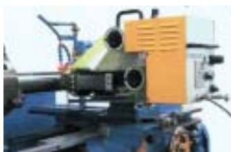
Microfinishing unit mounted on the tool post of a lathe.
