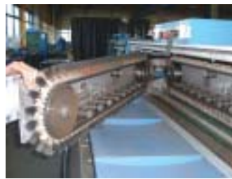
The wire brush endless belt as mounted on the machine
