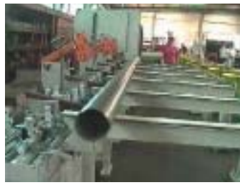
Multihead centreless tube finishing machines with automatic loading and unloading.
