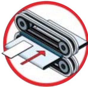
Drawing showing feed direction of conveyor and cross direction of abrasive belts.
