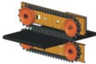
Diagram of deburring head with top and bottom abrasive flap belt
