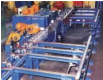
Multihead centreless tube finishing machines with automatic loading and unloading.
