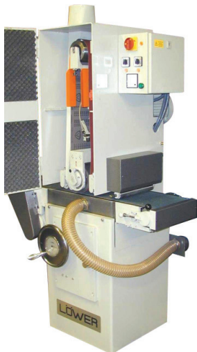
Model STN 300 with 1 abrasive belt head.
