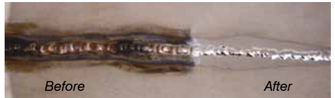
Before After Thermochemical Weld Polishing
