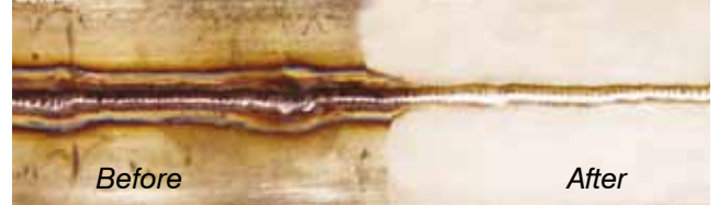
Before After Thermochemical Cleaning
