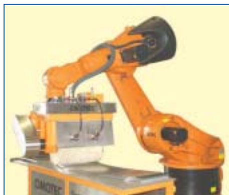
A robot with a wide buffing head polishing car trim
