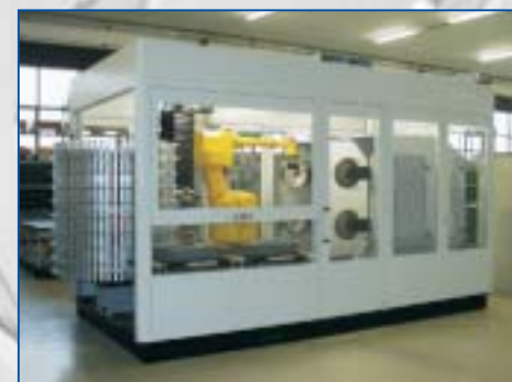
A typical robot cell in a booth and with rotary magazine
