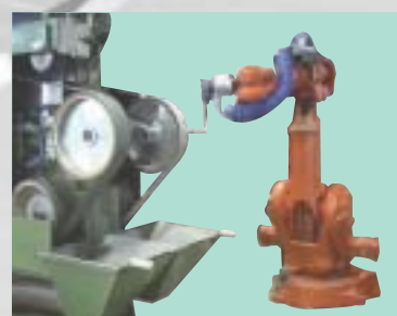
Linishing door handles
