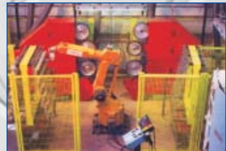
A typical linishing cell for sanitary fittings
