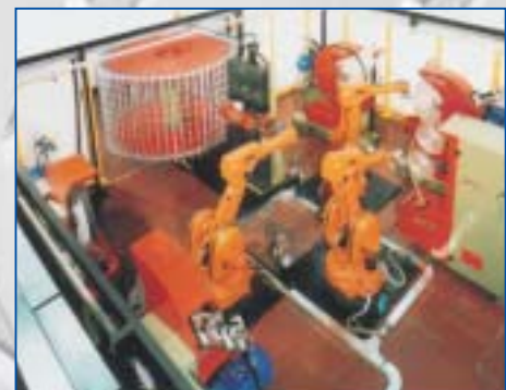
3 robots in a cell, linishing and polishing door handles
