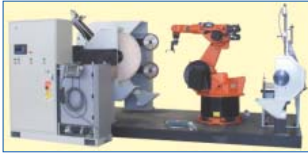
This shows the size of the central control cabinet in relation to the rest of the cell.
