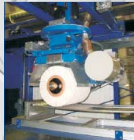
Longitudinal polishing of tubes
