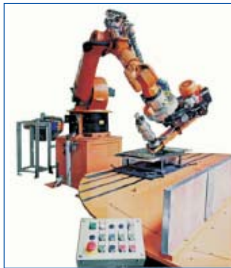
A robot with an internal brushing head polishes the inside of a stainless steel bowl
