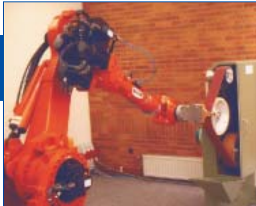
Grinding, deburring and finishing of a subframe
