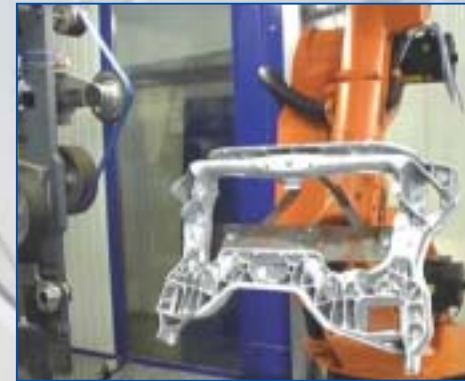
Grinding, deburring and finishing of a subframe
