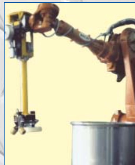
Grinding and polishing inside vessels
