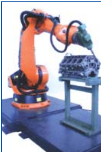
A robot with a special rotary tool head deburring an engine block
