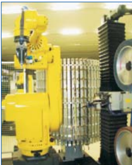
Robot on left, rotary magazine in the middle, pick and place arm on right.
