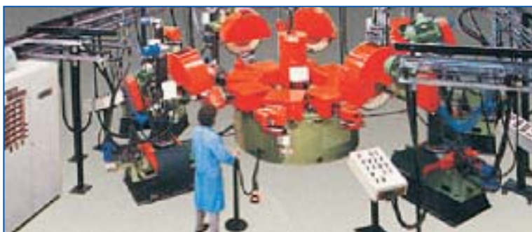
A typical robot cell in a booth and with pallet magazine
