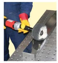
**Model SU** 110V 0r 240V, 2 HP, 2800 - 5800 rpm, max 150mm OD
