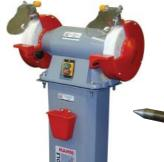
Medium duty bench polisher with an optional stand. Motor: 230V, 1.2 HP, 2900 rpm, max 200mm dia.
