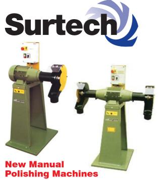
New machines have two speeds: 1400 and 2800 rpm. They are available single or double ended. With 1.7 - 2.3 HP motors. For greater versatility, they can be equipped with variable speed inverters.
