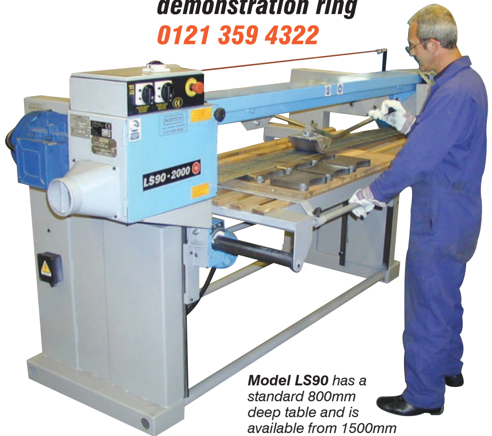
Horizontal belt for general purpose de-slugging, grinding and finishing.
