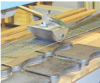
Horizontal belt for general purpose de-slugging, grinding and finishing.
