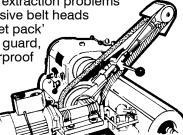
Wet operation means using water as coolant with a proprietary additive added to aid lubrication and prevent corrosion.
