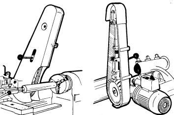
LEH abrasive belt head shown here with guard modified for both contact wheel and slack of belt grinding. Shown on left with belt tensioning lever. On right with access door removed to show internal tensioning and tracking controls.
