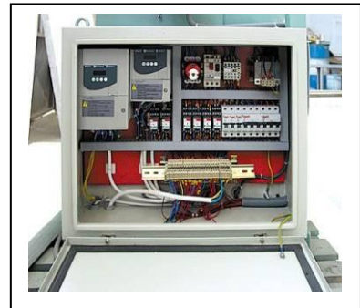
Above, The inside of a typical top of the range abrasive belt grinder
