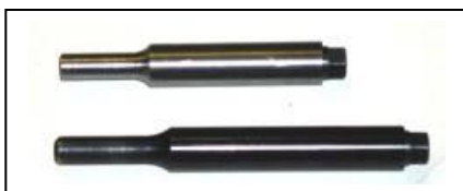
On the left: Collet extensions. Fit into standard collets
