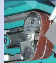
Special design abrasive belt head with oscillating contact rollers for producing a radius.
