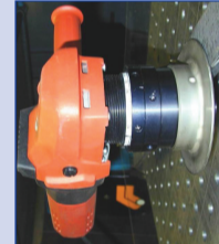
Portable chamfering machine. With milling cutters. Max bevel 12mm.
