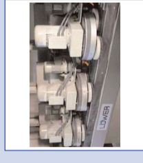
Two examples of planetary disc heads with multiple brushes.
