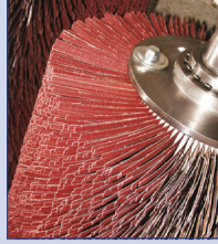
The type of abrasive rotary brush used in planetary rotary brush machines. Consists of slashed abrasive cloth.
