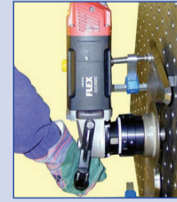
A portable radiusing machine with milling cutters to produce 2mm to 5mm radius.
