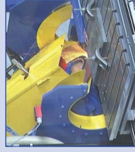
Abrasive belt chamfering / bevelling machine. Max bevel 40mm.
