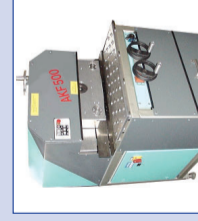
Extra heavy duty pedestal chamfering / bevelling machine.
